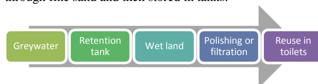
Fig 8: Greywater treatment process
