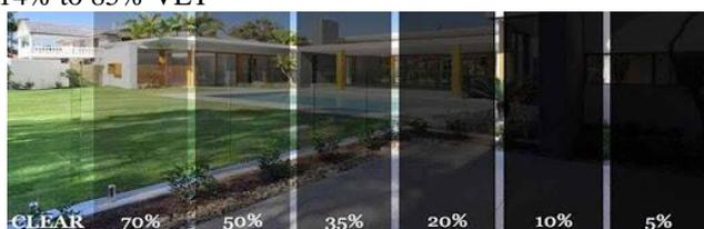
Fig 5: Comparison of glasses with different VLTs
