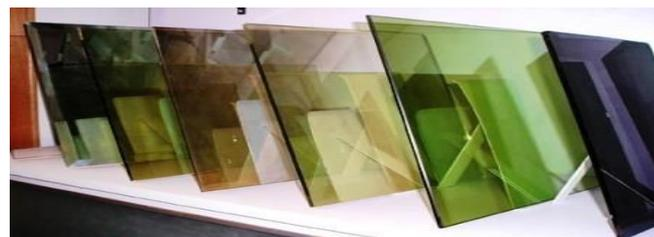
Fig 6: Tints of heat absorbing glass
