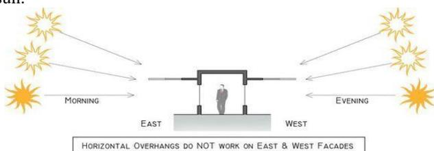
Fig 14: Shading Issues with East and West Facades
