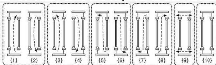
Fig 17: Airflow regimes in cavity
