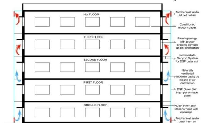
Fig 16: Cross section of a sample DSF
