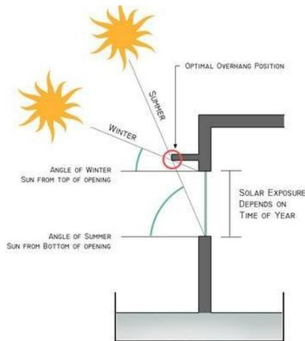
Fig 13: Basic Shading Strategy for a South Elevation
