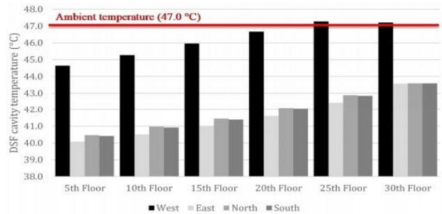
Fig 15: Sample simulation results showing average cavity temperature for each orientation and floor
