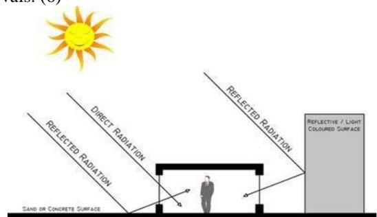
Fig 11: Sources of Solar Radiation that May Require Shading
